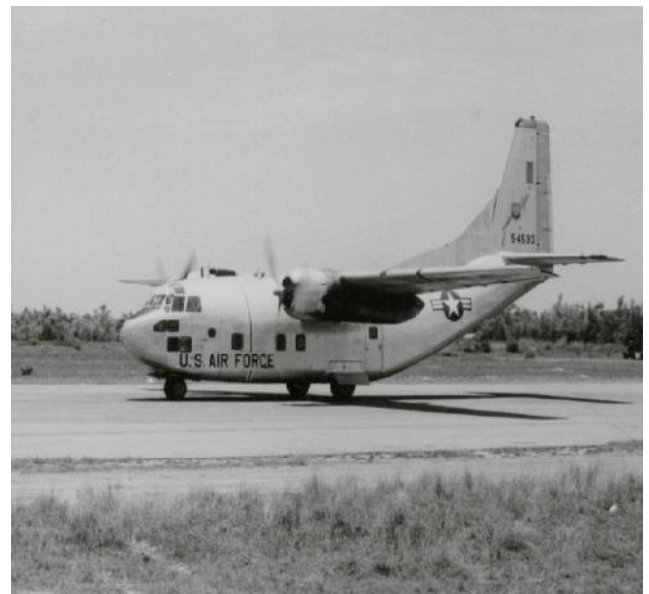
The Air Force C-123, was a smaller two-engine version of the C-130, used primarily for resupply missions to small, remote landing fields
