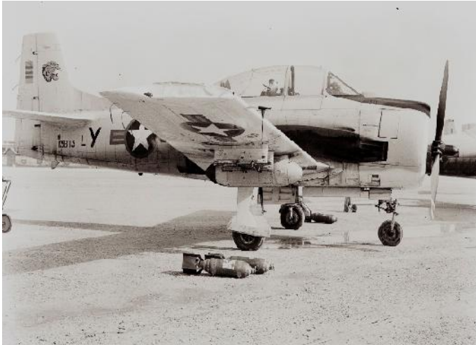
The T-28, used to train American military pilots since the early 1950's, had been e-configured as a combat aircraft for the Vietnamese Air Force. It had wing pylons that could carry bombs, napalm and rockets as well as 7.6 and 50 caliber machine guns.
