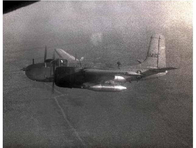
The Douglas B-26 Invader was a relic of the Korean war, that bristled with 50 caliber machine guns had Vietnamese Air Force markings and flew missions out of the Air Force side of the DaNang airbase.
